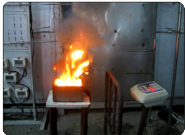
Fig 7.5.1: Pool Fire Experimental Facility for PFBR Turbine Oil
