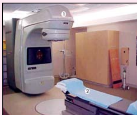
Fig.1: Medical Linear Accelerator (1-Linear Accelerator, 2 - the adjustable treatment couch)
