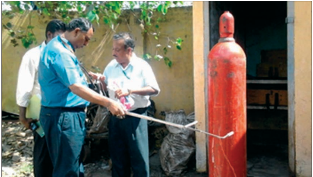
Demonstration using the Co 60 gamma gauge for CO 2 level measurement
